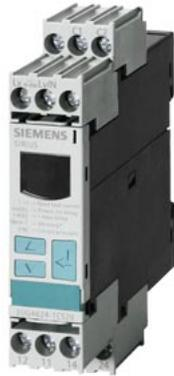
Digital monitoring relay for residual current monitoring (with converter 3UL22) Setting range 10-100% of transformer rated value separate for warning threshold and switch-off value 90 to 690 V AC 50...60 Hz AC ON delay and tripping delay 0.1 to 20 s Shutdown hysteresis up to 50% Warning hysteresis 5% fixed 2 change-over contacts with or without fault buffer screw terminal Successor product: 3UG4625-1CW30 with transformer 3UL23
