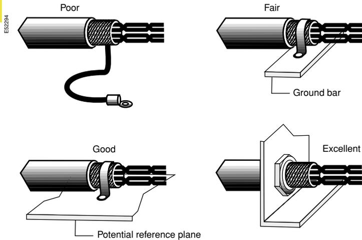
If a U-shaped clamp cannot be used to ground the shielding when connecting to a screw-type terminal, the grounding wire should be as short as possible. This type of connection should be avoided.
