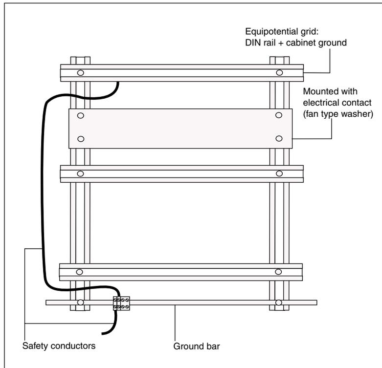
The presence of many equipotentially bonded structures in machines and cabinets provides maximum protection.
