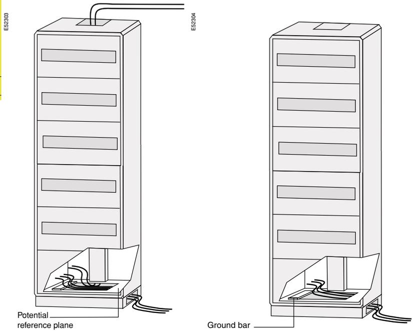
Equipotentiality must be guaranteed for cabinets placed side by side.
