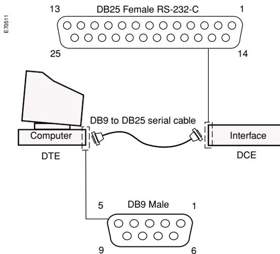
Some terminals and computers may have a DB9 type RS-232-C serial connector. In the figure above, the RS-232-C serial connection uses a DB9 to DB25 cable.
