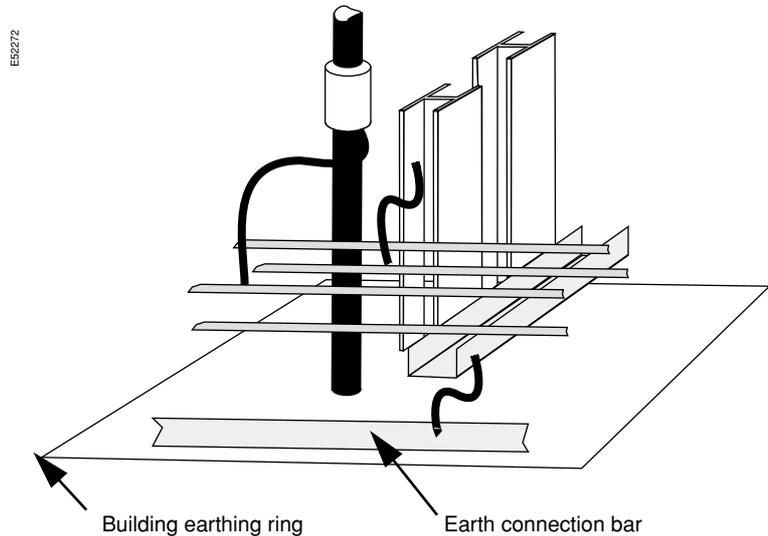
**Example of a grounding system for a building**
