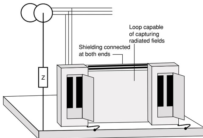
An initial insulation fault can lead to a phase-to-phase voltage between a phase conductor and the equipment ground. This is unacceptable for electronic devices supplied directly by a phase-to-neutral connection and which cannot withstand the phase-to-phase voltage.
