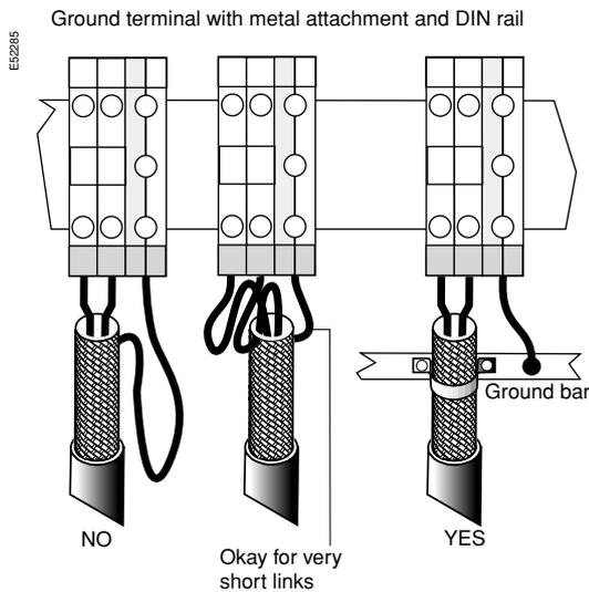
If a connector is used, it must provide a 360° electrical continuity between the cable shielding and the equipment ground.
