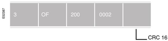
Returns the description of the type of controller at this address, the status of the "run indicator" and information specific to each type of slave. Broadcast not supported.
