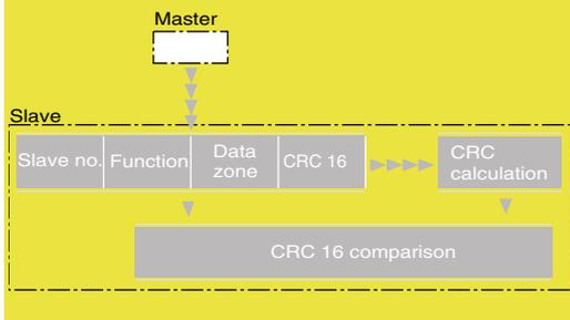
**Important:** the least significant byte (LSB) of CRC 16 is transmitted first.
