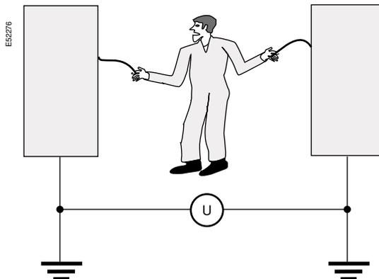
To ensure trouble-free operation of equipment and the safety of persons, all exposed conductive parts must be interconnected and earthed to ensure equipotentiality.
