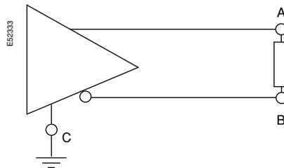
Line "A" on the transmitter is negative with respect to line "B" for a binary "1" (OFF).
