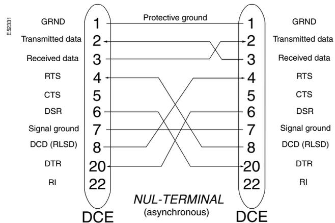
**Definition :** Flow control allows the receiver to order the terminal to stop transmission when its buffer memory has reached 90% of its capacity. There are two types of control: hardware and software.
