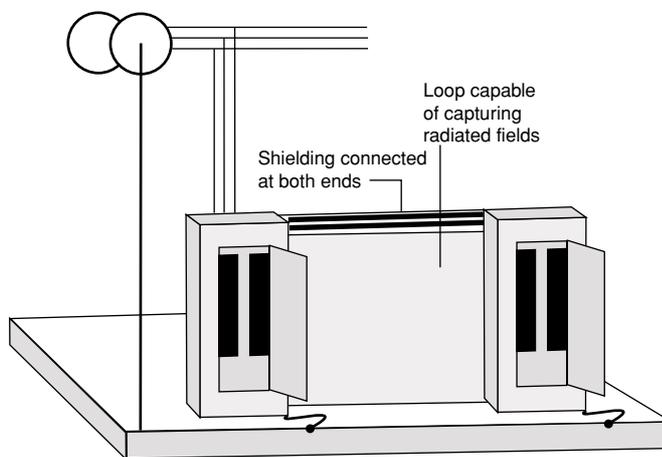
Note that overvoltages may be caused by separate earth electrodes for which the potentials vary differently.
