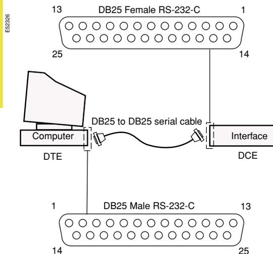
**Definition:** DTE (Data Terminal Equipment) represents the terminal or computer.
