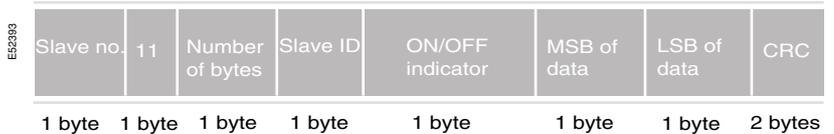
**Note:** The number of bytes, slave ID and data available depend on the type of slave. For the ON/OFF indicator: FF = ON & 00 = OFF.
