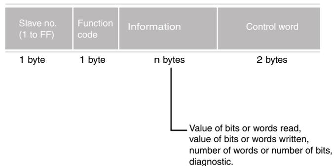
Each module has a single address on the network. This address is between 1 and 255 (1 and FF in hexadecimal).
