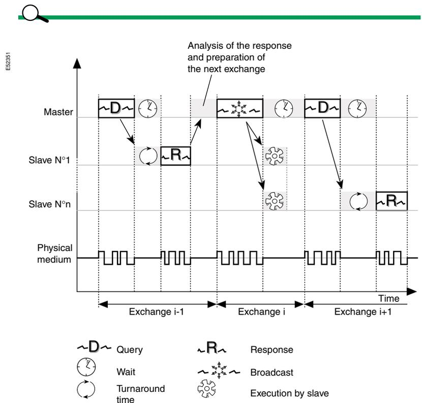
**Note:** The lengths of QUERY, RESPONSE, BROADCAST, WAIT and PROCESSING depend on the function performed.
