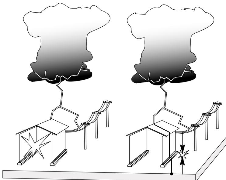
**Definition:** An exposed conductive part is an accessible metal part that is isolated with respect to the live parts of the equipment but which may accidentally become live.
